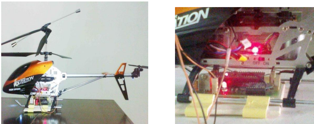
Fig-5 Sensor Package “CURIOUS”, along with GPS installed in an RC copter.
